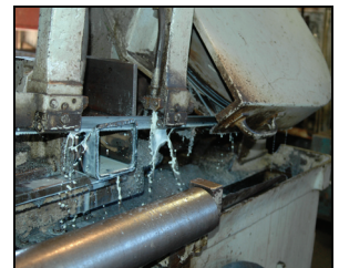
A Marvel, 16" hydraulic horizontal band saw, cutting 6"x6" sq. tube.
