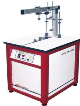
The 3000 shaper carves profiles in turned or arced shapes—from a 24" diameter column base to intricate gothic arch and 'S' curves.
