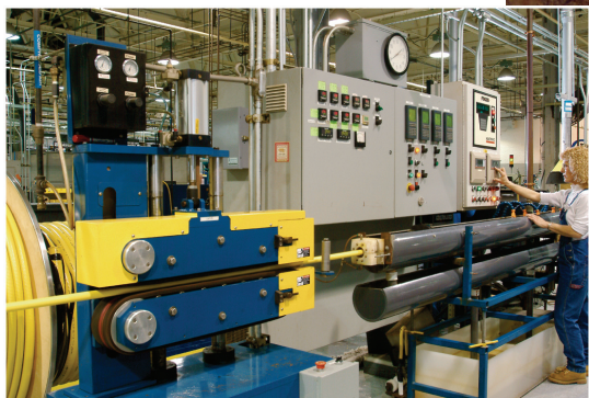
Automated, computer-controlled machines encase corrugated, stainless steel tubing in a polyethylene jacket.
