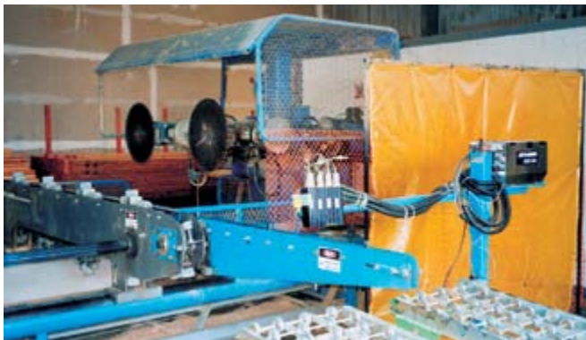
The Koskovich Auto-Omni saw also is equipped with a Jet-Mark printer so information about each job can be printed as required on the members as soon as they are cut. The printer even works on wet wood.
