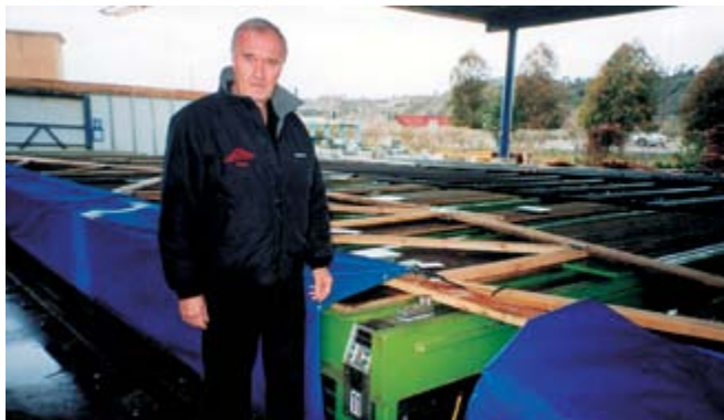
Sartor stands near one of the computer-controlled Jet-Set installations for patterning trusses. Because table is in a typical California wall-less plant, tarps are used to cover the system during rain storms.
